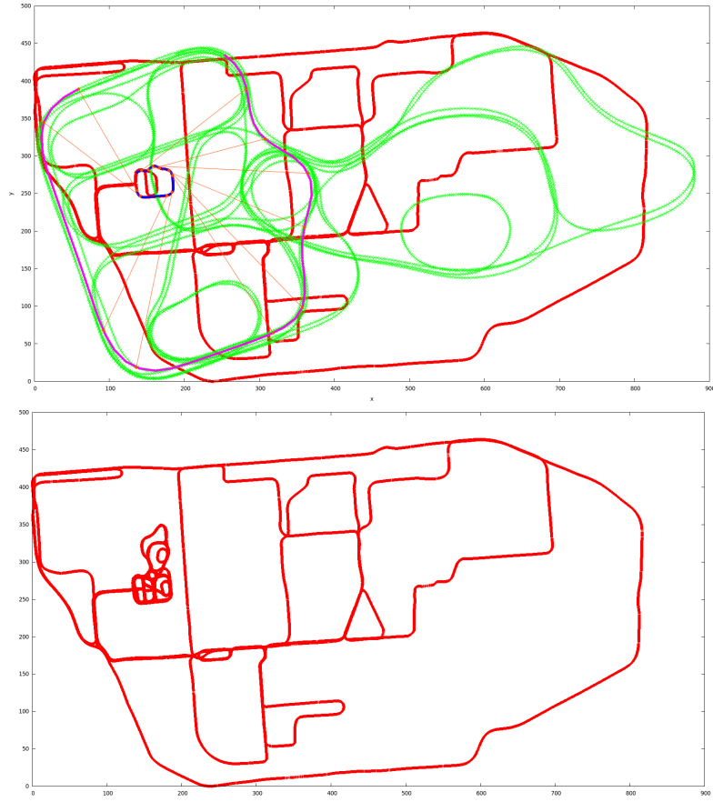
Fig. 4: Path merging from two paths with different scale and frame of reference. Purple and blue parts are common segments found. Orange lines shows the rigid transformation. The result of the merging is shown on the second figure.
